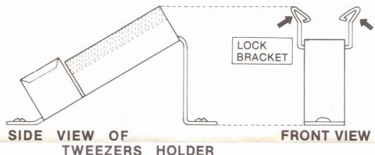
HOTWEEZERS® will lock into place when properly returned to it's holder, making it impossible for the tweezers to be accidentally bumped or shaken loose.
